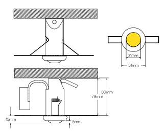
Cut out size: 40-43mm Ambient operating temperature 30°C
