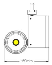
For dimentions C/W potentiometer add 20mm to height of fitting Ambient operating temperature 25°C
