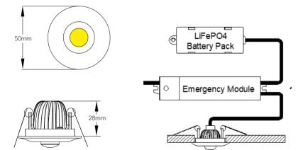
Cut out size : 40mm Ambient operating temperature 30°C
