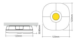
Cut out size : 40-43mm Ambient operating temperature 30°C
