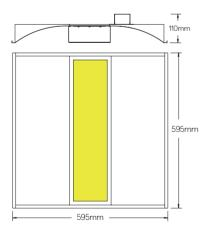
Ambient operating temperature 25°C - Do not cover back of fitting
